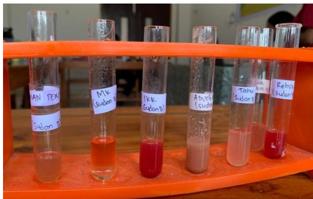
Figure 5 Fat test results using the Sudan III test
