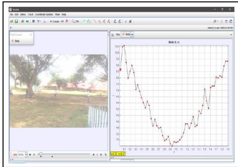
Figure 3 Video analysis using tracker software for parabolic motion
