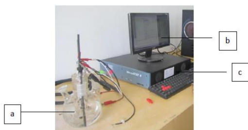
Figure 2. A set of corrosion rate testing tools (a. testing tube, b. monitor, c. potentiostat)
