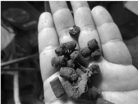
Gambar 2. Produk Pellet Sampah PLTU Co-Firing
