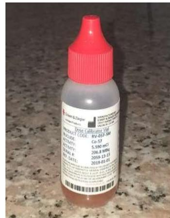
**Gambar 5. Sumber standar radionuklida Co-57**
