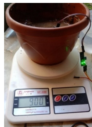
Figure 5 Calibration process of YL 69 sensor
