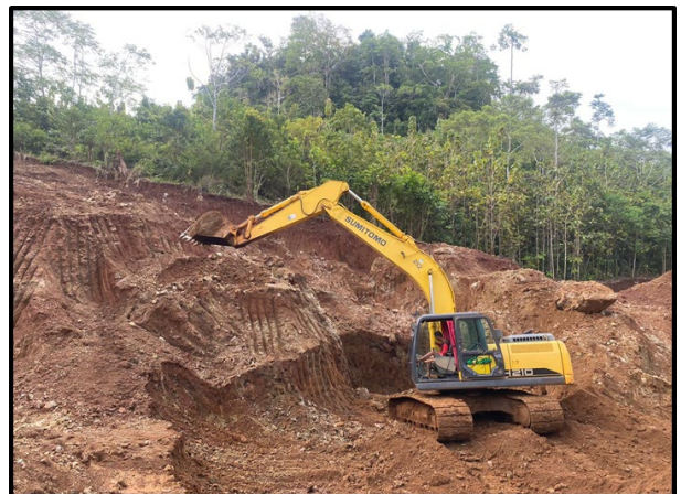
Gambar-10. Proses ore getting
