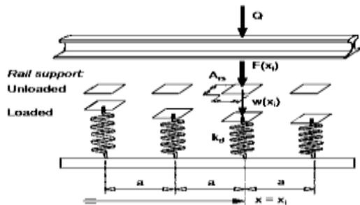
Figure 3. Discrete elastic support model.<sup>3</sup>
