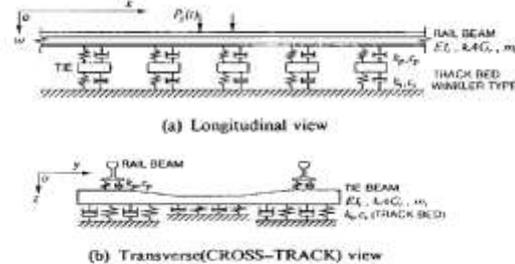
Figure 4. The idealized rail track/beam system.<sup>4</sup>
