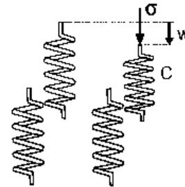
Figure 1. Winkler support model.<sup>1</sup>
