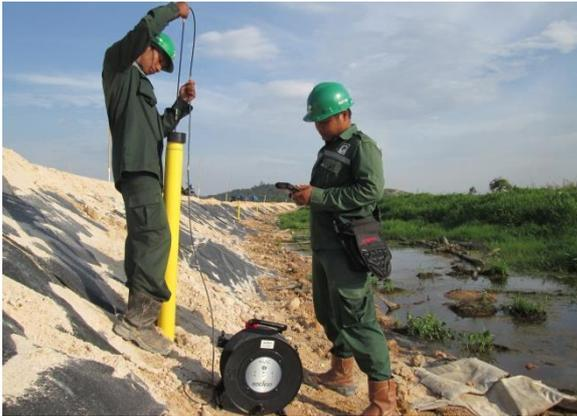
Gambar 52. Monitoring inclinometer
