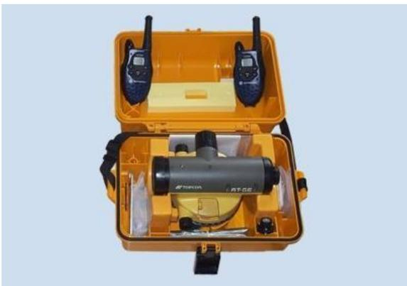
**Gambar 41.** Alat monitoring *settlement plate*
