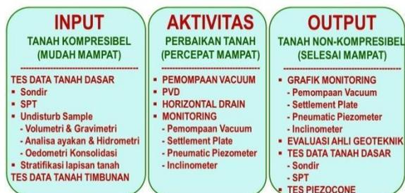
**Gambar 15.** Proses *vacuum consolidation*
