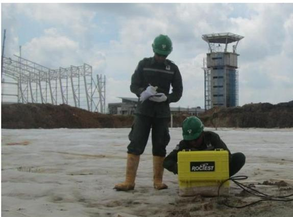
Gambar 47. Monitoring *pneumatic piezometer*
