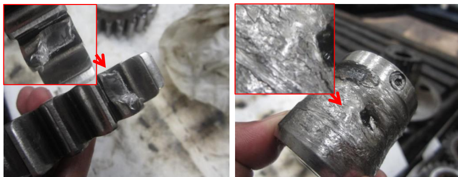
Gambar 12. Cleavage Planet Gear & Dimple Rupture Pin
