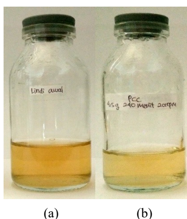
Figure 3. Leachate (a) before adsorption and (b) after adsorption using PCC
