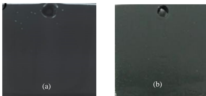
Figure 2. (a) Iron surface with a blank layer (C), (b) Iron surface with a superhydrophobic silica layer (SS1).
