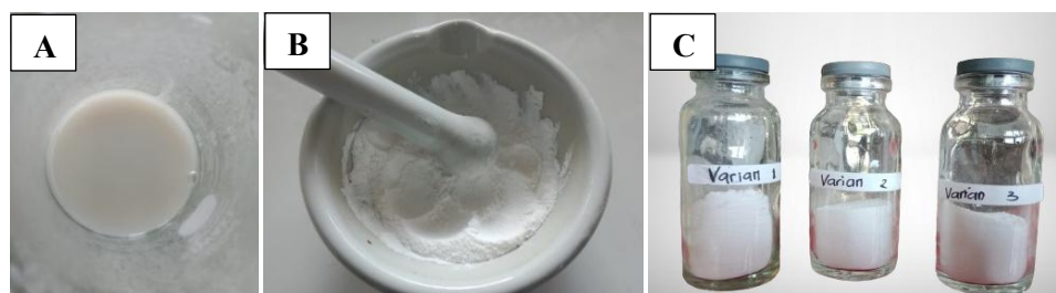
Figure 4. (a) Silica functionalization process with triethanolamine, (b) Grinding of the synthesized fluorescent silica, and (c) Fluorescent silica variants 1, 2, and 3 that have been ground.
