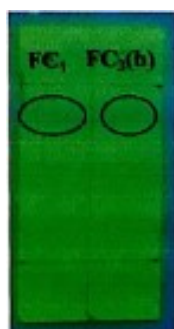
Figure 4. FC1 and FC2(b) TLC chromatograms, viewed under UV light at 254 nm, the stationary phase was Silica Gel TLC GF254, the mobile phase was n-hexane:chloroform TLC (1:1)
