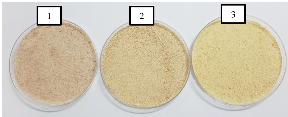
Figure 2. Difference Colour of Glucomannan Extract; (1) Extraction Using Multilevel Concentration of Ethanol; (2) Extraction Using Fixed Concentration of Ethanol; (3) Iles-iles Kuning Flour
