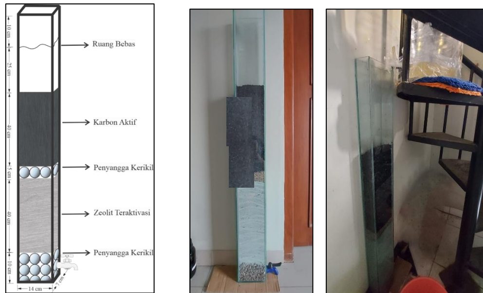
Gambar 2. Reaktor Filtrasi-Adsorpsi Percobaan
