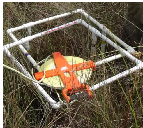
Figure 2. Quadrat and other apparatus used for understory necro mass and diversity.
