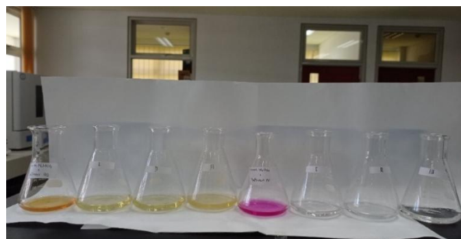
Figure 5. Color Changes at the Endpoint of NaHCO 3 -HCl Titrations
