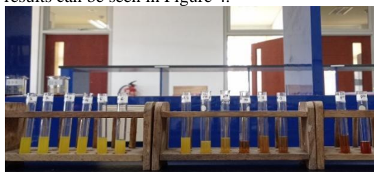
Figure 4. Color changes of extract in pH 1- 14 Buffer Solution
