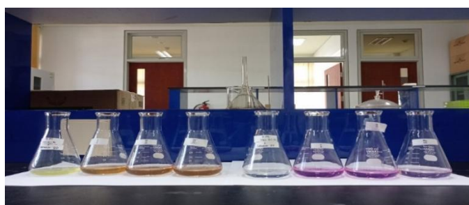
Figure 4. Color Changes at the Endpoint of HCl-NaOH; CH 3 COOH-NaOH Titrations
