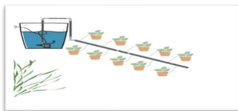
Figure 1 Design of fertigation system installation
