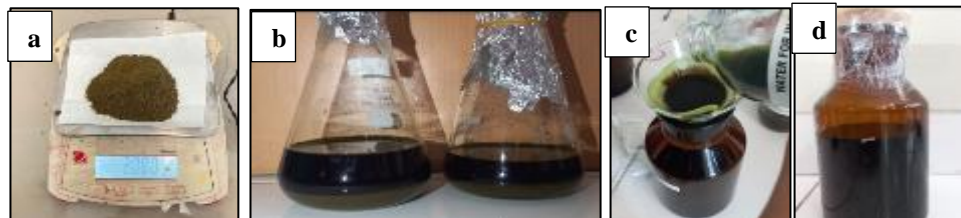
Figure 4 Maceration procedure (a) Weigh the powdered betel leaf, (b) Mix the powder with ethanol in a bottle and let it stand for three days, (c) Perform maceration, and (d) Result of maceration (macerate)
