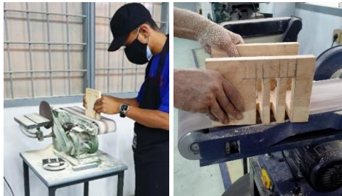
Figure 4 Using an emery mill to smooth the wood surface
