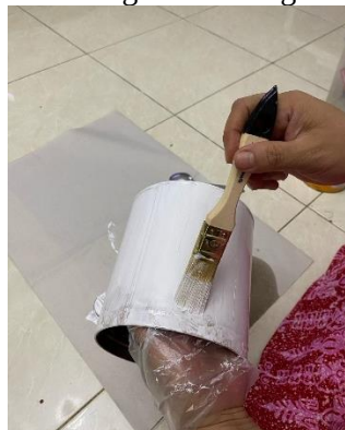
Figure 5 Base coat application process
