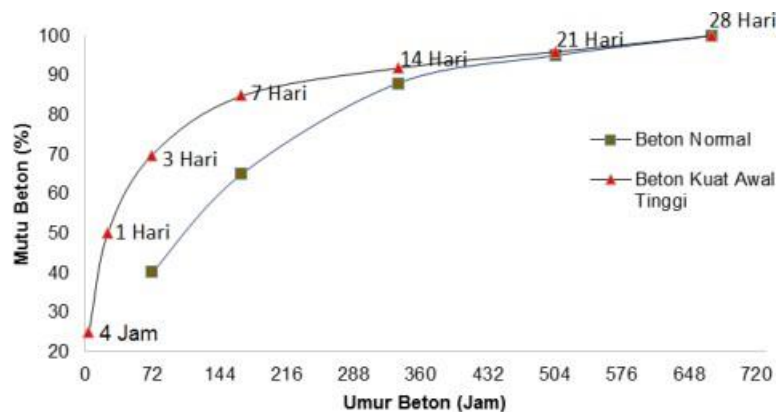
Figure 2. 1 Graph of age compared with the percentage of concrete (PBI, 1971 and SHRP, 1993)
