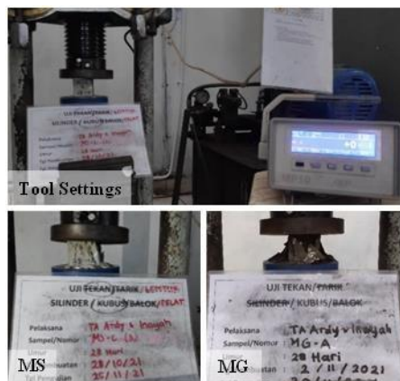
Figure 30 Compressive Strength Test of Mortar
