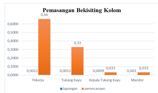
Figure 4. 2 Comparison Chart of Column Formwork Installation Coefficient Value
