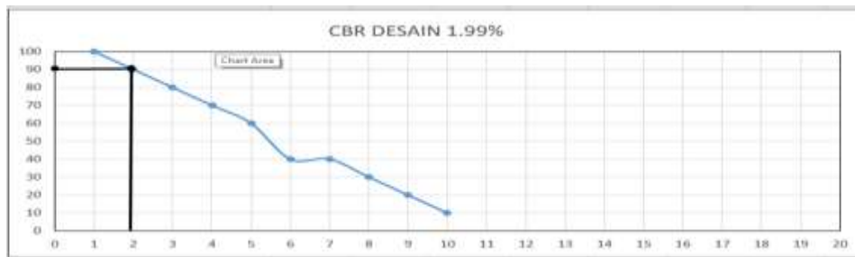
Figure 4.1 Relationship Graph subgrade CBR value with Graphic Method
