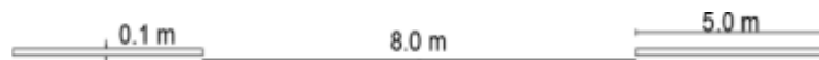
Picture 7. Placement of Longitudinal Marking and Median Substitution Double Lines Side View
