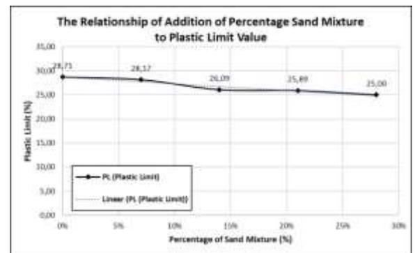
Figure 8. Graph of Relationship of Addition of Percentage of Sand Mixture to Plastic Limit Value
