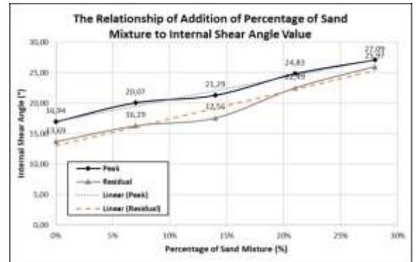
Figure 5. Graph of Relationship of Addition of Percentage of Sand Mixture to Internal Shear Angle Value
