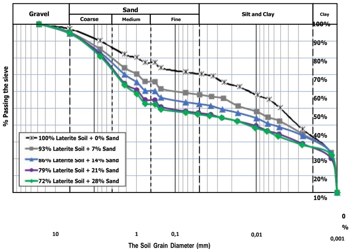
Table 4. Results of Analysis of Grain Size Distribution of Laterite Soil with Mixed Sand
