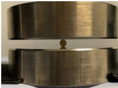
Figure 1. Specimen During DTS Test
