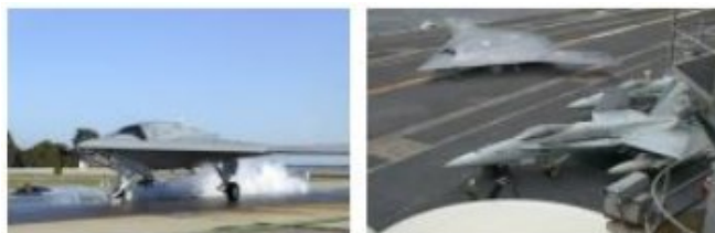
Figure 15. X-47B PTTA UCAV type with stealth technology is in trials for landing and fly on an aircraft carrier.
