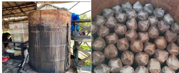
Gambar 6. Baglog disterilisasi didalam drum
