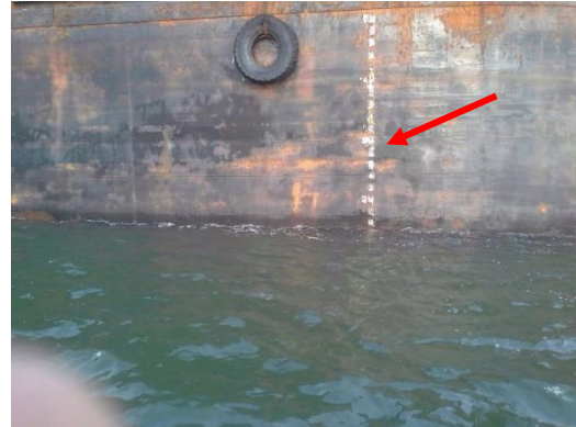
Gambar-3. Draft Tongkang / Vessel
