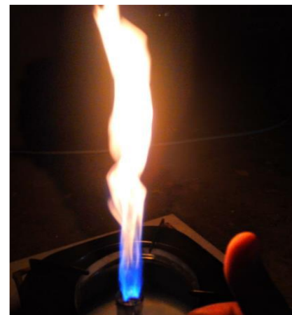
Figure 4 Gas Stove is Ignited using The Pertamina Fuel
