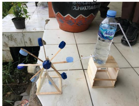
Figure 2 A simple project applying Bernoulli's law
