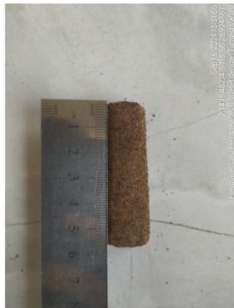
Gambar 3. Biopellet Daun Jati ( Tectona grandis )
