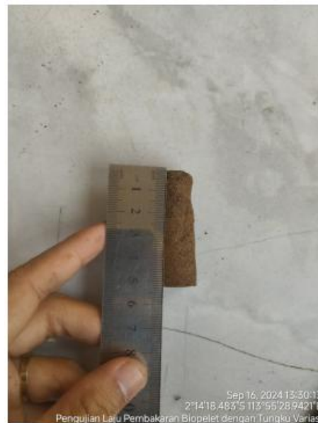
Gambar 2. Biopelet daun Sirsak ( Annona muricata )
