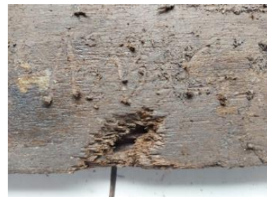
Gambar 11. Hasil Serangan Marine Borers
