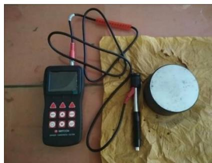
Gambar 4. *Portable Hardness Tester Digital*
