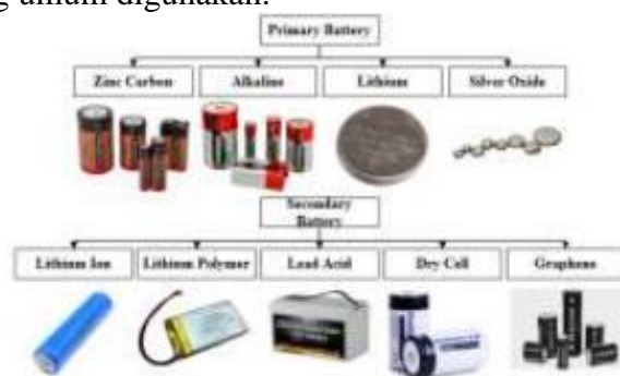
Gambar 3. Primary dan Secondary Battery
