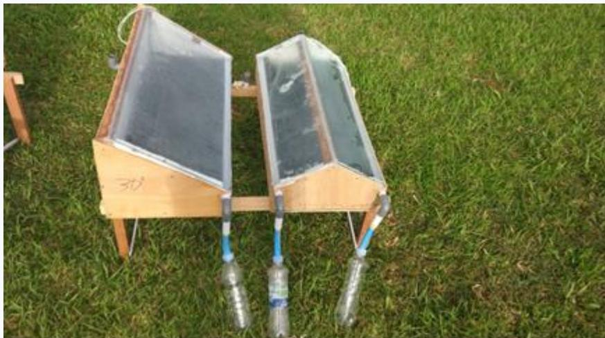
Gambar 1. *Solar Distillation*
