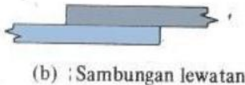
Gambar 2. Sambungan Lap joint
