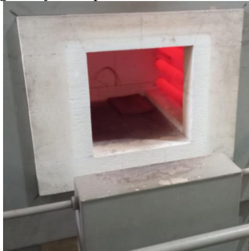
Gambar 3. Proses Post Weld Heat Treatment
